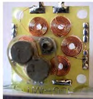
D. Spremann et al., 2006 HSG-IMIT 260 \mu\text{W} , 4 m/s 2 @ 25 Hz, 1.5 \text{cm}^3
