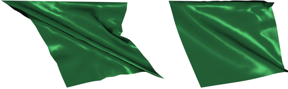
Figure 8: Two configurations of a sheet fixed at the top and pulled from the bottom right corner. Left: triangle strain; right: edge strain.
