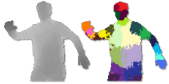
Fig. 4. Depth map and labeled body segments of the upper torso.
