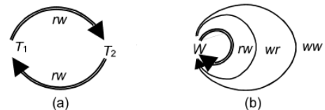
Fig. 2. SDG and DSG for write skew example
