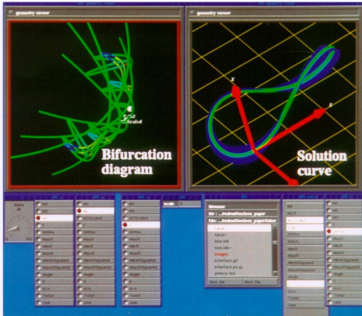
Fig. 1. The PCR interface shows the bifurcation diagram projection (on the left) and the solution projection (on the right). The GUI at the bottom allows the user to select both projections.
