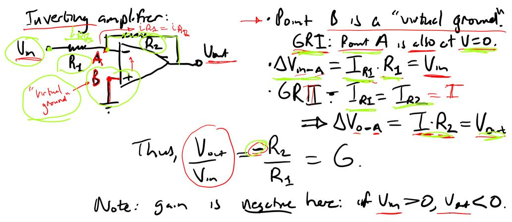
What is the input impedance of this amplifier? (hint: it is <u>not the input impedance of the op-amp!</u>)
