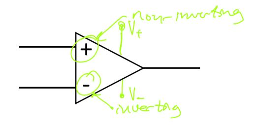
\* The typical op-amp (e.g. the LE411) has an open-loop gain of  $10^5 - 10^6$
