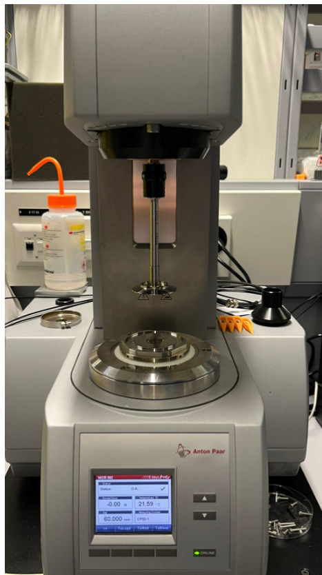
Figure 1. Rheometer used for the measurements
