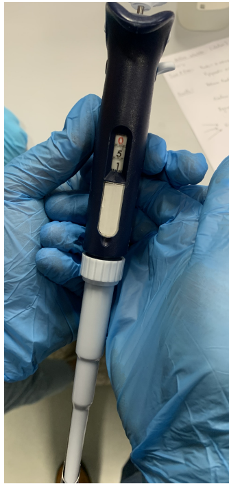
Figure 3: Display Window of P1000 Micropipette. The numbers specified on the window correspond to a volume of 510 \mu L .
