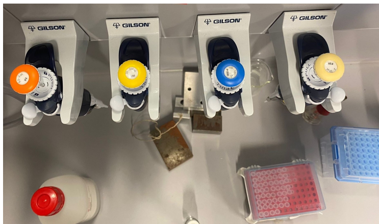
Figure 1: Micropipette Set in the Lab. The micropipettes available in the lab are of sizes: P2, P20, P200, and P1000.
