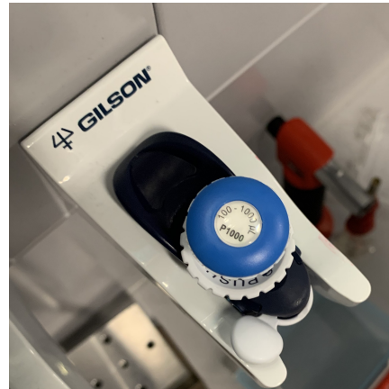
(a) Operational Volume Ranges for Different Pipette Sizes. The nominal size of a variable-volume pipette is the maximum volume that can be carried by this pipette. (b) P1000 Micropipette. This micropipette can hold volumes within: 100 - 1000 \mu\text{L} .
