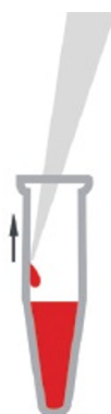
Figure 6: Side Wall Expelling. This figure shows the process of expelling extracted liquid while the tip touches the host container side wall to make sure all needed volume is reached [6].
