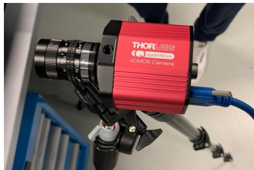
Figure 2: Camera used for DIC Analysis. The camera used in the experiment was a Quantalux 2.1 MP Monochrome sCMOS Camera from THORLABS.
