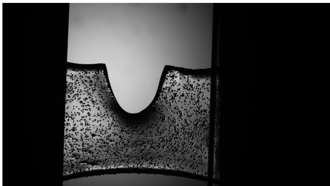
(a) Before crack propagation
