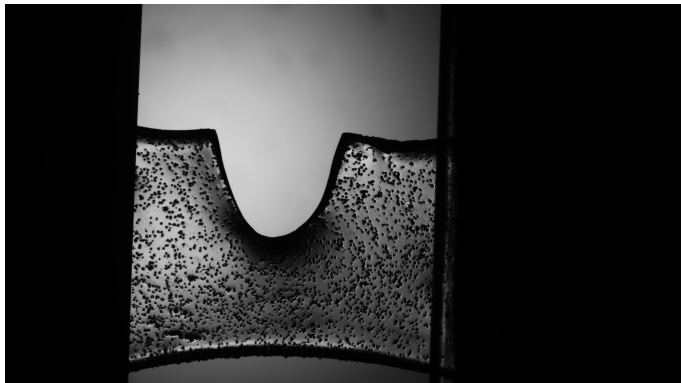
(b) After crack propagation
