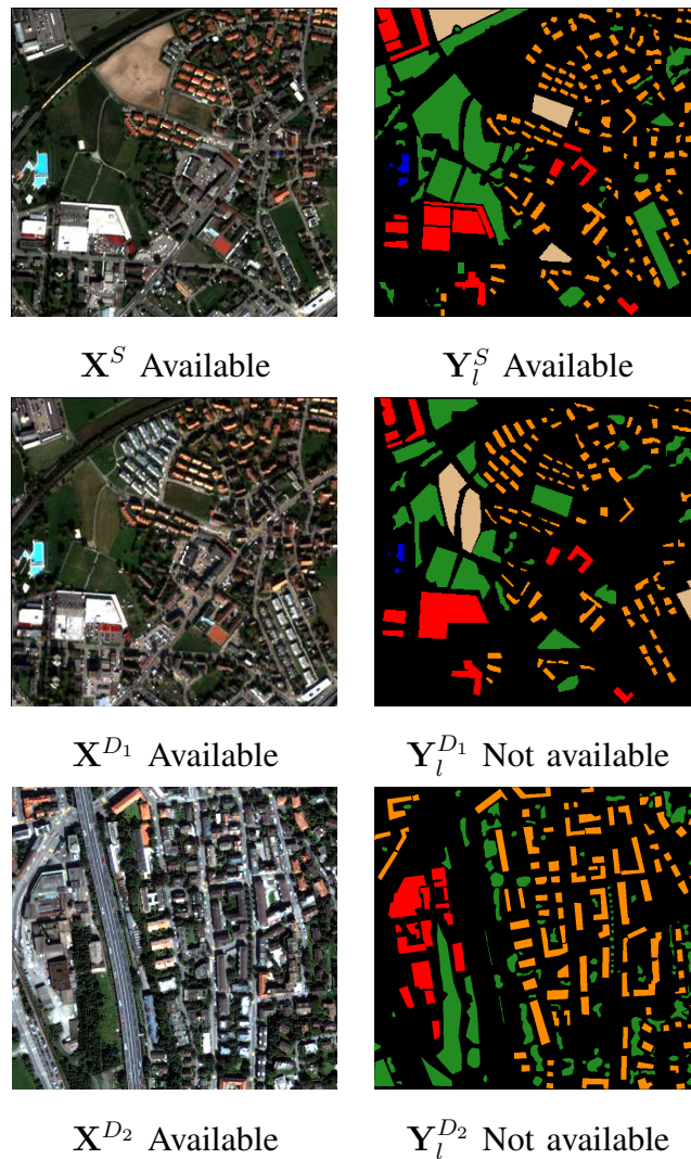
Fig. 1. Illustration of the domain adaptation problem. Source image \mathbf{X}^S (top) and the same kind of objects, destination images, taken at a different time ( \mathbf{X}^{D_1} middle) and at a different time and location ( \mathbf{X}^{D_2} bottom). The right column shows the respective labeled pixels (colors are detailed in Table I). Note that \mathbf{Y}_l^{D_1} and \mathbf{Y}_l^{D_2} are usually not available and are used here only for validation purposes. Details on the images are given in Section III-B.
