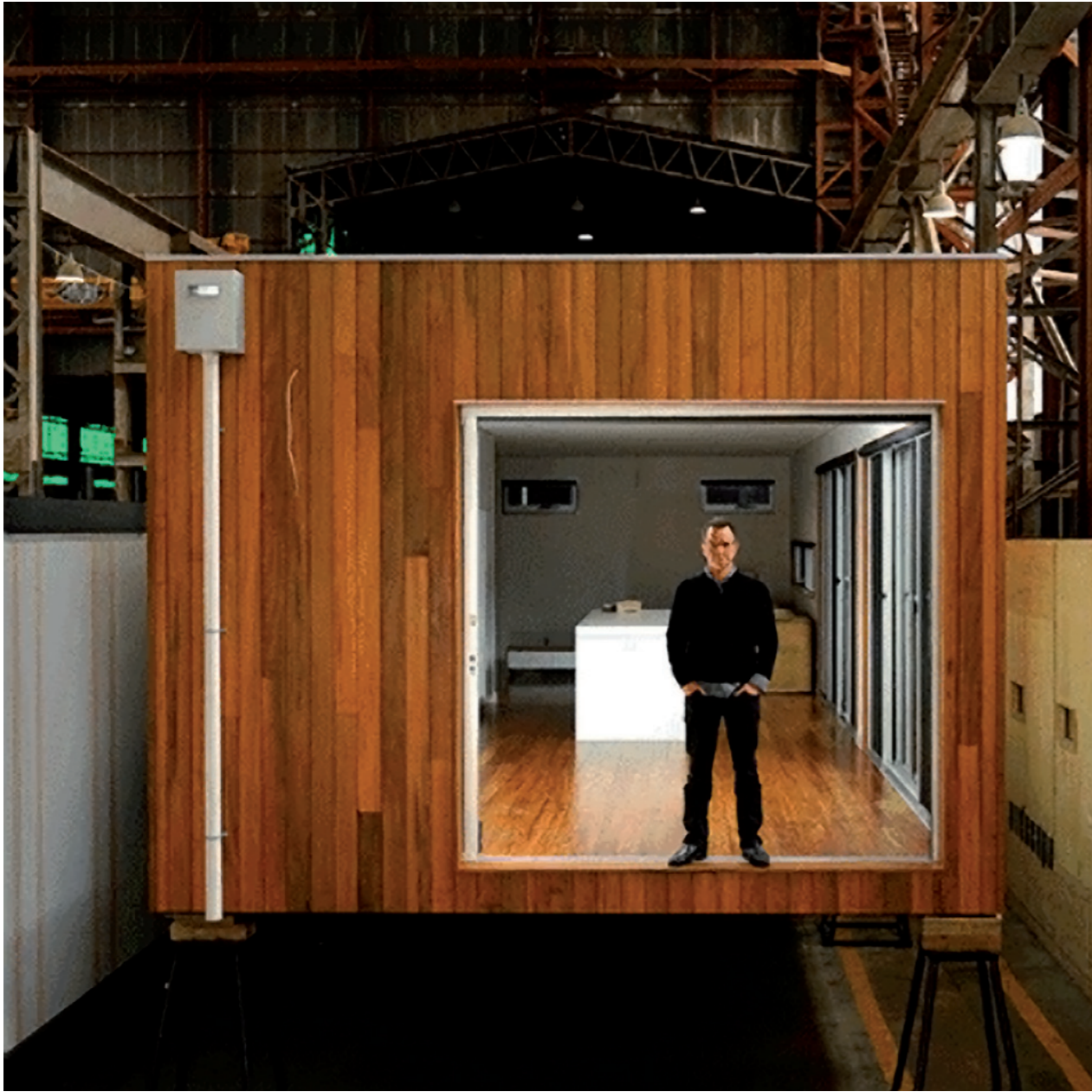
A «pre-build» module apartment made by Modscape that could possibly be adapted to high rise
