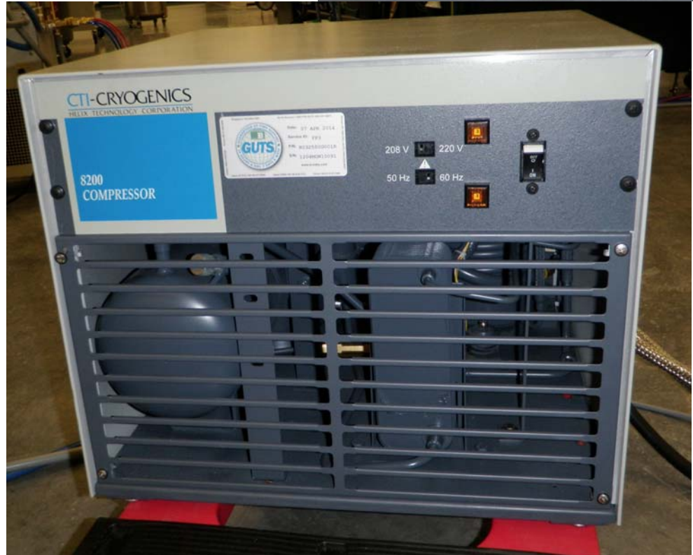
220V/208V Switch on Cry-Compressor
