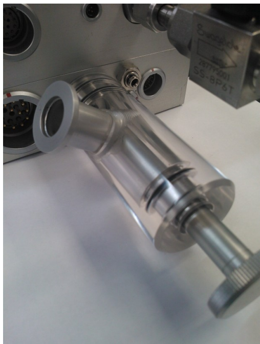
(c) To pump on the VTI vacuum space, use this adapter. Pull back the plunger, fit the cylinder over the valve, screw the plunger into the valve, then pump out the cylinder before pulling back the plunger to open the valve.
