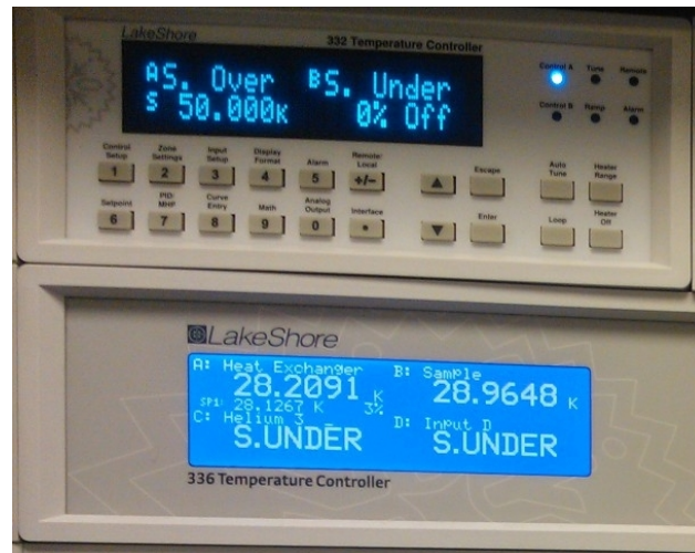
(a) Lakeshore temperature controllers displaying thermometer readings. The upper controller (332 or 335) displays the temperatures of the main and mini sorbs on the ^3\text{He} probe (chapter 10). The lower controller (336 or 340) displays the VTI thermometers A (heat exchanger) and B (sample), see chapter 3.1.4, and the ^3\text{He} probe sample temperature. Sensor D on the 336/340 is the voltage across the pressure transducer in the ^3\text{He} probe gas chamber.
