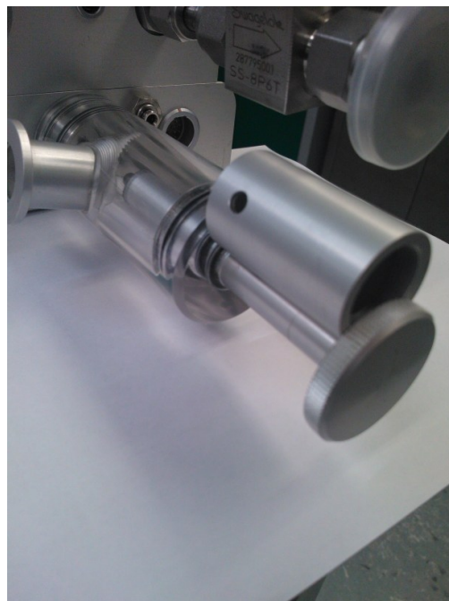
(d) The vacuum inside the VTI will pull the valve closed but it can easily be held open, e.g. with the valve cover as shown.
