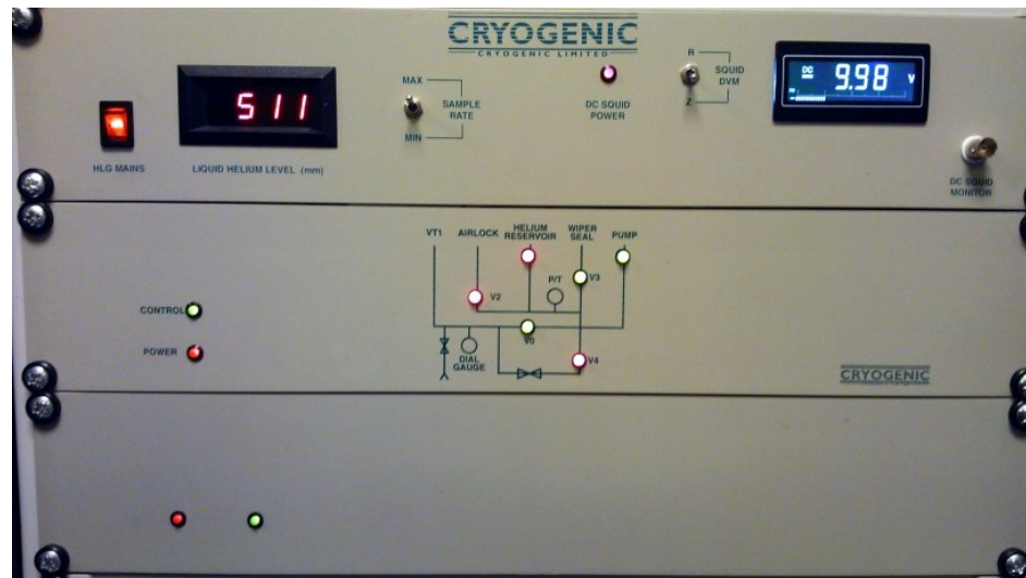
(b) Front panels of the Helium level gauge, SQUID output meter and Data Acquisition system (DAQ). The DAQ front panel shows the status of the valve block. Red and green LEDs show the state of valves and pumps, green for open/on and red for closed/off.
