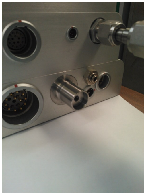
(b) This is the pumping port for the VTI vacuum space.
