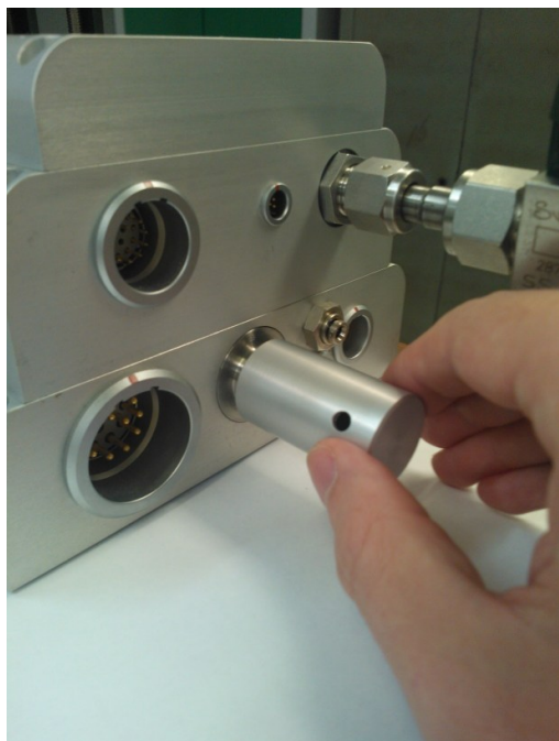
(a) When not pumping via this port the cover should be screwed in place to catch the blow-off valve in the event it blows off.
