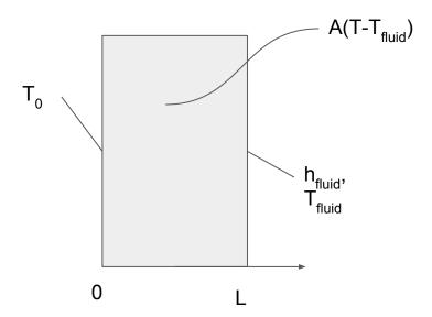
$$\frac{\partial^2 T}{\partial x^2} + \underbrace{\frac{\partial^2 T}{\partial y^2} + \frac{\partial^2 T}{\partial z^2}}_{= 0, \text{ since}} + \underbrace{\frac{\dot{q}}{k}}_{= 0, \text{ since}} = \underbrace{\frac{1}{\alpha} \frac{\partial T}{\partial t}}_{= 0, \text{ since steady}}$$
