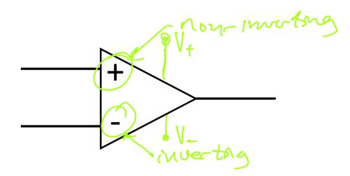
\* The typical op-amp (e.g. the LF411) has an open-loop gain of  $10^5$  -  $10^6$
