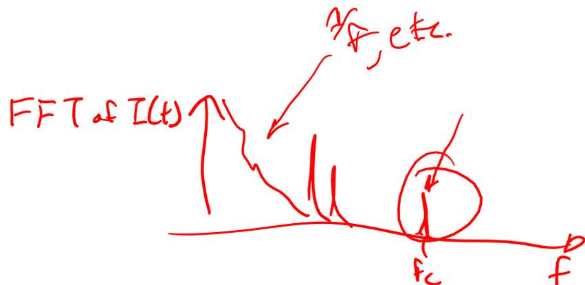
chop Ph.D. } → × } →  $\int_0^{\Delta T} I(t) \cdot \sin(2\pi f_c t) dt$  } → DC level, Ampl. @  $f_c$ .
