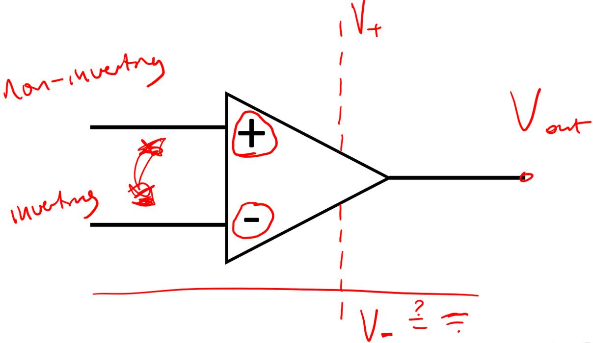
\* The typical op-amp (e.g. the LF411) has an open-loop gain of 10<sup>5</sup> - 10<sup>6</sup>
