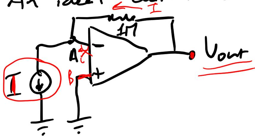
This circuit produces an output of  $1\text{V}/\mu\text{A}$  of current: useful for e.g. a photodiode, which makes current when exposed to light.
