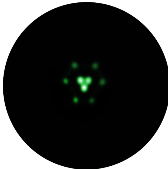
Fig. 1. The FIM pattern for the ALIS He ion source.
