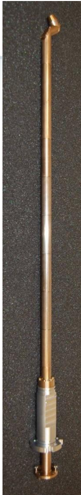
Inside NMR probe: 8 mm waveguide
